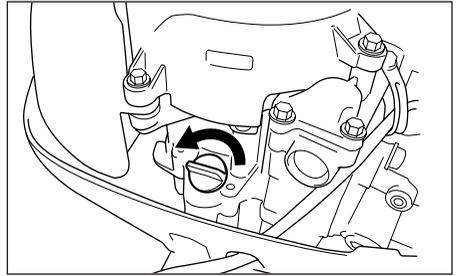
3. Place a drain pan under the engine oil drain plug.
