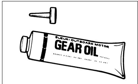
Use SUZUKI OUTBOARD MOTOR GEAR OIL, or an equivalent high quality SAE90 hypoid gear oil.
