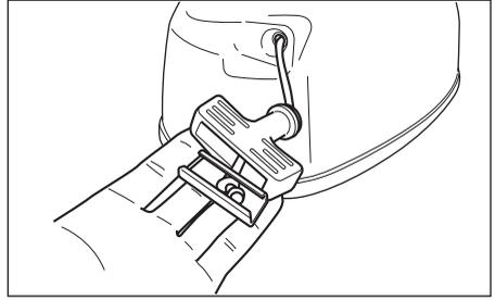
5. Install the handle grip back to the end of rope.
