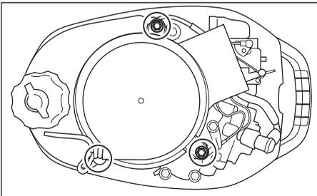
4. Lift off the recoil starter assembly.
