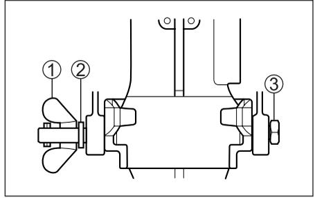
4. Reposition the tilt pin in the desired holes.
