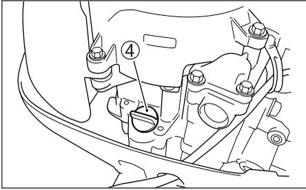
3. Fill the recommended engine oil to the upper level.
