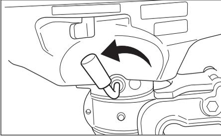
5. The lock plate (A) is in place and the end of the lanyard is attached to a part of your body.
