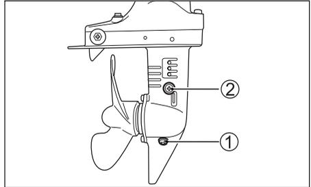
3. After the oil has drained completely, inject the specified gear oil into the lower drain hole until it just starts to come out of the upper hole. Approximately 60 ml (2.0/2.1 US/lmp oz.) of oil will be required.
