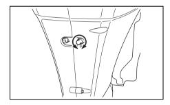
4. Ensure that the boat fuel tank is correctly vented and that any in-line filters are free of dirt etc. If fuel tank filler cap has a manual vent, be sure that it is fully open.
