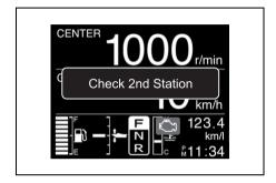
The "Check 2nd Station" indication clears when any of the button is pressed in the gauge. However, the caution alarm icon is displayed until eliminating the cause.
