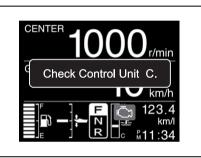
The "Check Control Unit C." indication clears when any of the button is pressed in the gauge. However, the caution alarm icon is displayed until eliminating the cause.
